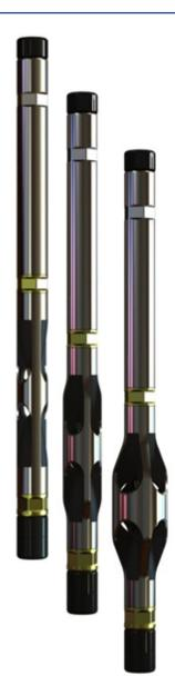
The In-Line Flowmeter (IFM001,002,004) is a compact inline tool that provides a continuous flowmeter log while in tubing and can provide a secondary/back up flowmeter to the Full Bore or Fixed Cage Spinners whilst logging in casing or liners. Available in 3 sizes from 1.69-3.15" OD, it is robust, reliable and simple to service.
