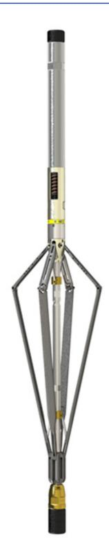
The XY Caliper Tool (XYC002) provides a continual measurement of independent X & Y internal tubular diameters by means of measurement arms set at 90° apart. The tool closes to 1.69" and opens to 9.00" allowing use in both tubing and casing up to 9-5/8" OD.
